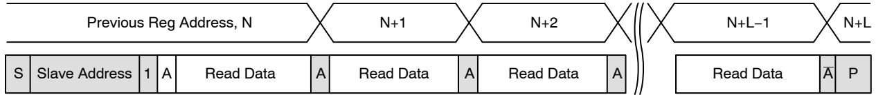
Figure 13. Sequential READ, Start from Current Location
