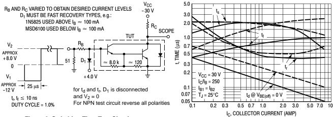
Figure 2. Switching Time Test Circuit
