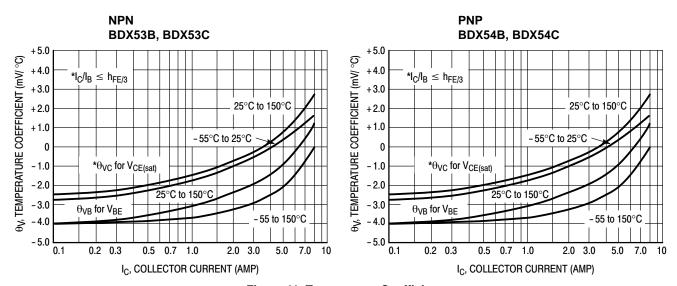
Figure 11. Temperature Coefficients
