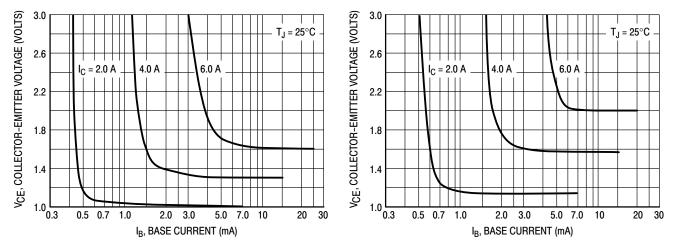
Figure 9. Collector Saturation Region
