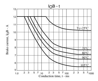
STK681-352-E Allowable Brake Current Range (High side: F1, F2=ON) or Allowable Startup Current Range
