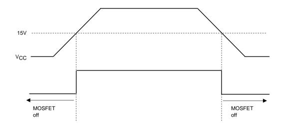
When  $V_{CC}$  < 15V, an internal control voltage has not risen above the preset threshold level, so ENABLE must be set to low in order to turn off the MOSFET.
