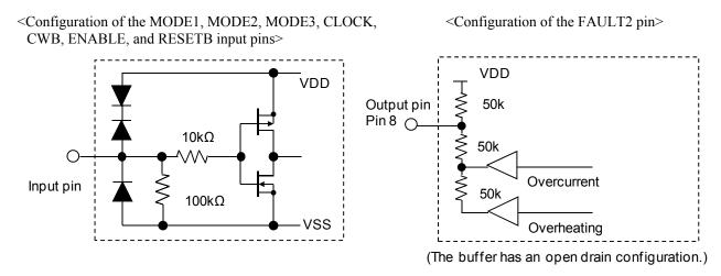
The input pins of this driver all use Schmitt input. Typical specifications at Tc=25°C are given below. Hysteresis voltage is 0.3V (VIHa-VILa).
