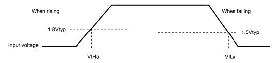
Input voltage specifications are as follows.  $V_{IH}$ =2.5Vmin  $V_{IL}$ =0.8Vmax
