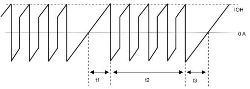
Motor COM Current Waveform Model
