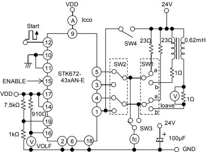
Ioave measurement : Set switch SW2 in the setting SW1 to 'b'. fc measurement : Set switch SW3 in the setting SW1 to 'a'. Icco measurement : Set ENABLE low.
