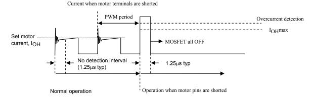
Overcurrent detection begins after an interval of no detection (a dead time of  $1.25\mu s$  typ) during the initial ringing part during PWM operations. The no detection interval is a period of time where overcurrent is not detected even if the current exceeds I<sub>OH</sub>.
