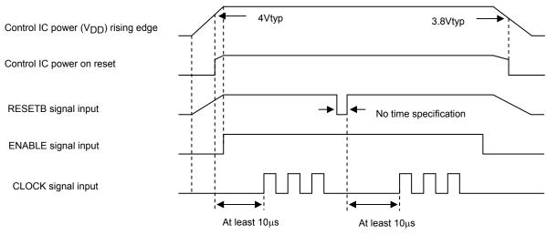
ENABLE, CLOCK, and RESETB Signals Input Timing
