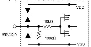
The input pins of this driver all use Schmitt input. Typical specifications at Tc=25°C are given below. Hysteresis voltage is 0.3V (VIHa-VILa).
