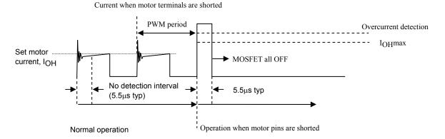
Overcurrent detection begins after an interval of no detection (a dead time of 5.5µs typ) during the initial ringing part during PWM operations. The no detection interval is a period of time where overcurrent is not detected even if the current exceeds I<sub>OH</sub>.
