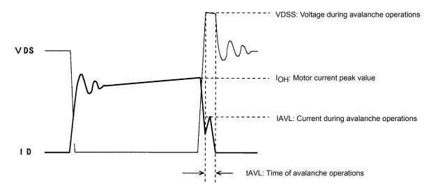
Figure 1 Output Current, ID, and Voltage, VDS, Waveforms 1 of the STK672-6\*\* Series when Driving a 2-Phase Motor with Constant Current Chopping
