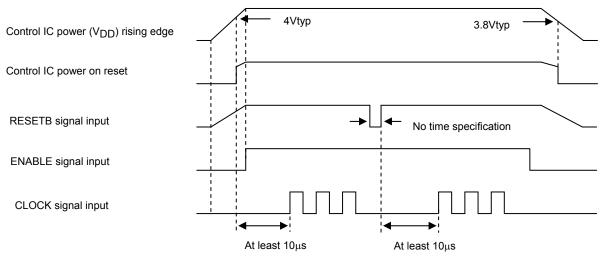
ENABLE, CLOCK, and RESETB Signals Input Timing
