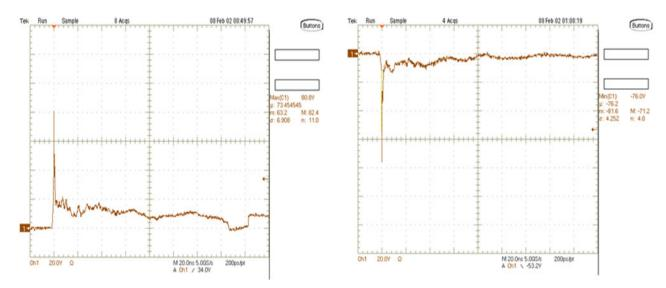
Figure 1. ESD Clamping Voltage Screenshot Positive 8 kV Contact per IEC61000-4-2
