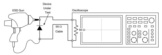
Figure 10. Diagram of ESD Test Setup
