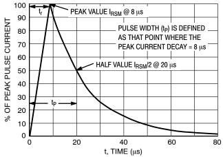
Figure 11. 8 X 20 µs Pulse Waveform
