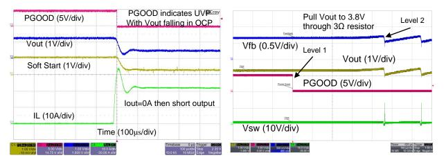
Figure 22. Over-Current Protection with Heavy Load Figure 23. Over-Voltage Protection Level 1 and Level 2
