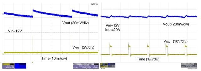
Figure 16. Static Load Ripple at No Load
