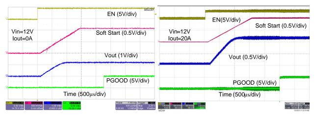
Figure 12. Startup Waveforms with 0 A Load Current Figure 13. Startup Waveforms with 20 A Load Current
