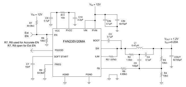
Figure 1. Typical Application with  $V_{\text{IN}}$  = 12 V
