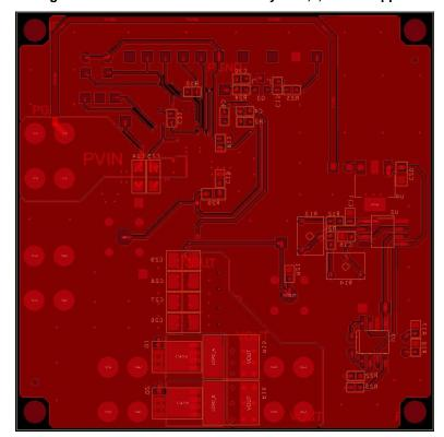
Figure 27. Evaluation Board Bottom Layer Copper
