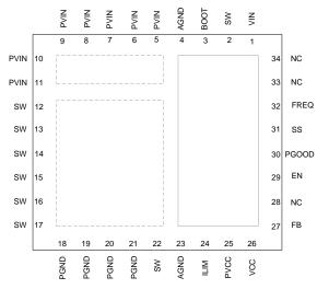
Figure 4. Pin Assignments, Bottom View
