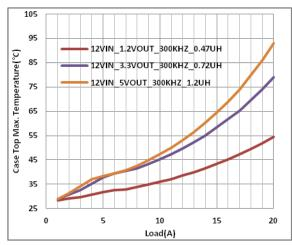
Figure 8. **Case Top Temperature vs. Load Current** with V<sub>IN</sub>=12 V and f<sub>SW</sub>=500 kHz
