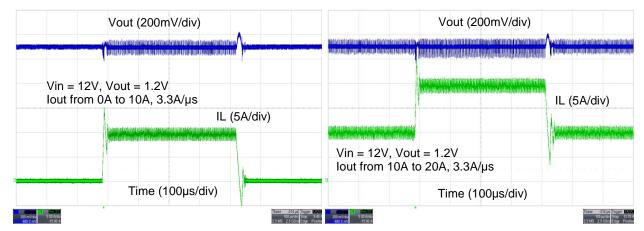
Figure 20. Load Transient from 0% to 50% Load Current
