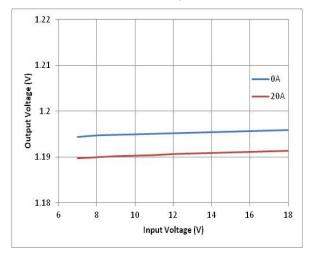
Figure 10. Load Regulation with VIN=12 V, VOUT=1.2 V Figure 11. Line Regulation with VIN=12 V, VOUT=1.2 V and fsw=500 kHz
