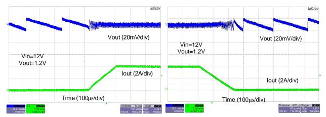
Figure 18. Operation as Load Changes from 0 A to 2 A
