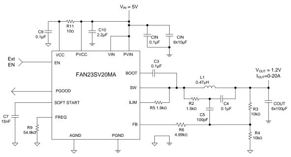
Figure 2. Typical Application with V<sub>IN</sub>=5 V
