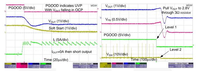
Figure 24. Over-Current Protection with Heavy Load Figure 25. Over-Voltage Protection Level 1 and Level 2
