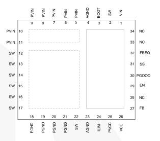
Figure 5. Pin Assignments(Top View)
