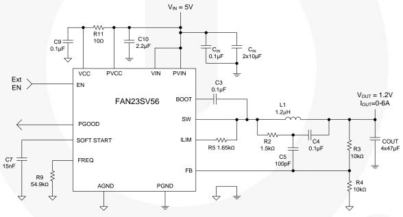
Figure 2. Typical Application with V<sub>IN</sub>=5 V
