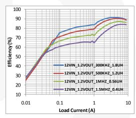
Figure 8. Efficiency vs. Load Current with  $V_{\text{IN}}$ =19 V and  $V_{\text{OUT}}$ =1.2 V
