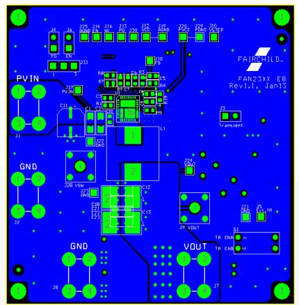
Figure 26. Evaluation Board Top Layer Copper
