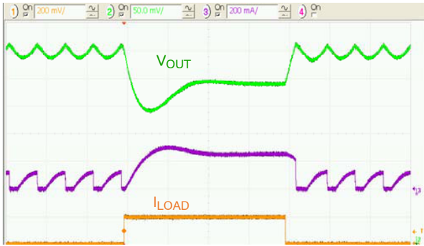
图 23. 负载瞬态, 50 mA 至 250 mA, V_{IN} = 3\text{ V} , t_{RISE} = t_{FALL} = 100\text{ ns} , 5\text{ }\mu\text{s/div} .
