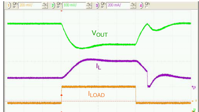
图 24. 负载瞬态, 150 mA 至 400 mA, V_{IN} = 3\text{ V} , t_{RISE} = t_{FALL} = 100\text{ ns} , 5\text{ }\mu\text{s/div} .
