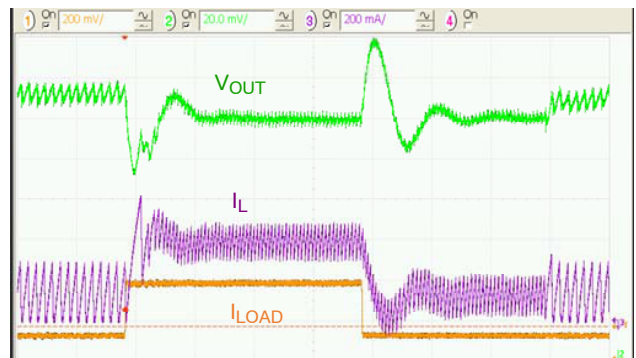
图 22. 负载瞬态, 150 mA 至 400 mA, V_{IN} = 3.6\text{ V} , t_{RISE} = t_{FALL} = 100\text{ ns} , 5 \mu\text{s}/\text{div} .
