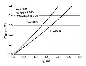
Figure 2. Conduction Voltage Drop Variation with Load Current.
