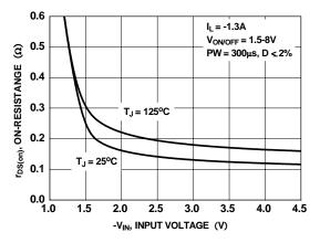
Figure 5. On-Resistance Variation With Input Voltage
