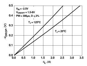
Figure 3. Conduction Voltage Drop Variation with Load Current.
