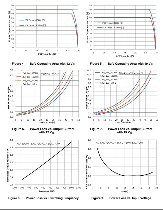
Test Conditions:  $V_{IN}$ =12 V,  $V_{CC}$ =P $V_{CC}$ =5 V,  $V_{OUT}$ =1 V,  $L_{OUT}$ =250 nH,  $T_A$ =25°C and natural convection cooling, unless otherwise noted.
