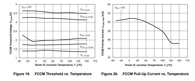
Test Conditions: VIN=12 V, VCC=PVCC=5 V, VOUT=1 V, LOUT=250 nH, TA=25°C and natural convection cooling, unless otherwise noted.
