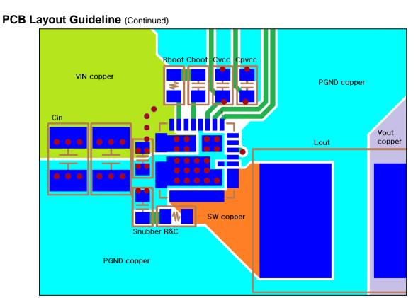
Figure 30. Single-Phase Board Layout Example – Top View
