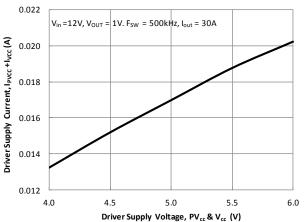
Figure 13. Driver Supply Current vs. Driver Supply Voltage
