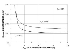
Figure 3. On-Resistance Variation with Temperature.
