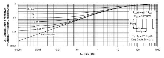
Figure 11. Transient Thermal Response Curve.
