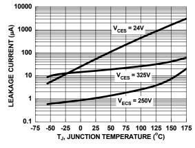
Figure 11. Leakage Current vs. Junction Temperature
