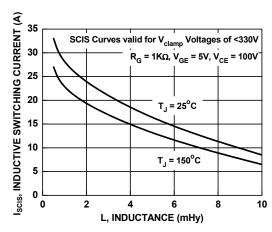
Figure 2. Self Clamped Inductive Switching Current vs. Inductance
