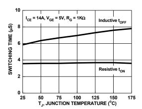
Figure 12. Switching Time vs. Junction Temperature
