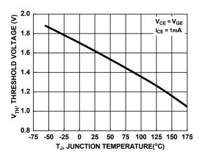
Figure 10. Threshold Voltage vs. Junction Temperature
