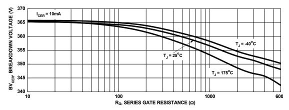
Figure 15. Break down Voltage vs. Series Gate Resistance
