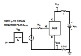
Figure 19. Energy Test Circuit
