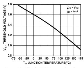
Figure 10. Threshold Voltage vs. Junction Temperature
