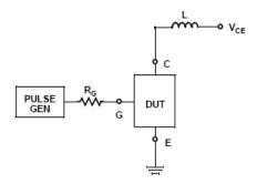
Figure 17. Inductive Switching Test Circuit
