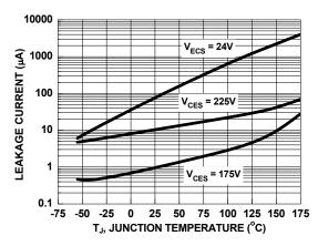
Figure 11. Leakage Current vs. Junction Temperature
