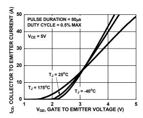
Figure 8. Transfer Characteristics
