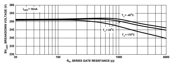
Figure 15. Break down Voltage vs. Series Gate Resistance
