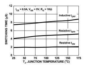
Figure 12. Switching Time vs. Junction Temperature
