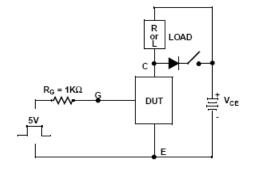
Figure 18.  $t_{\mbox{\scriptsize ON}}$  and  $t_{\mbox{\scriptsize OFF}}$  Switching Test Circuit
