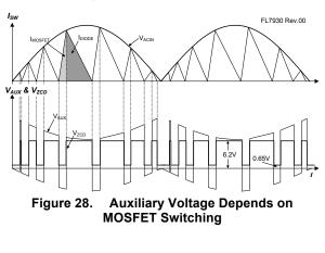
FL7930C — Single-Stage Flyback and Boundary-Mode PFC Controller for Lighting
