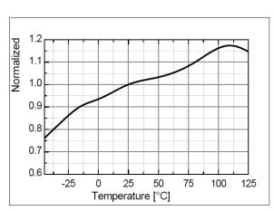
Figure 17. Output Voltage Low (VoL) vs. TA
