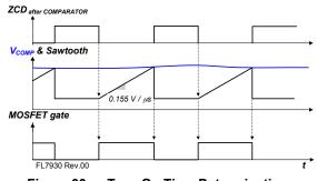
Figure 33. Turn-On Time Determination
