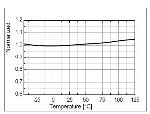
Figure 11. Maximum On-Time Program 1 (t<sub>ON,MAX1</sub>) vs. T<sub>A</sub>
