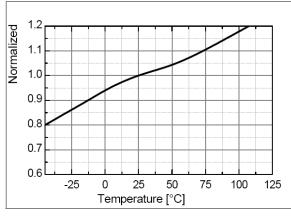
Figure 20. Output Saturation Voltage (V<sub>RDY,SAT</sub>) vs. T<sub>A</sub>
