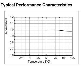
Figure 16. Output Voltage High (VOH) vs. TA
