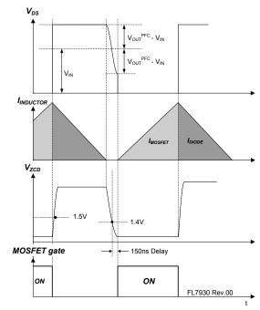
Figure 29. Auxiliary Voltage Threshold
