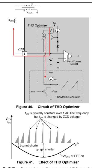
By THD optimizer, turn-on time over one AC line period is proportionally changed, depending on input voltage. Near zero cross, lengthened turn-on time improves THD performance.
