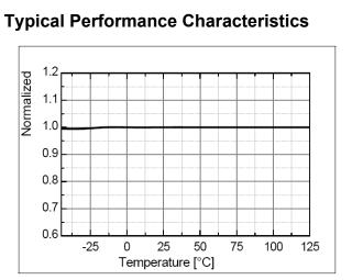
Figure 10. Zero Duty Cycle Output Voltage (V<sub>EAZ</sub>) vs. T<sub>A</sub>
