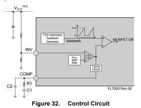
Unlike a conventional voltage-mode PWM controller, FL7930C turns on the MOSFET at the falling edge of ZCD signal. The "ON" instant is determined by the external signal and the turn-on time lasts until the error amplifier output ( $V_{COMP}$ ) and sawtooth waveform meet. When load is heavy, output voltage decreases, scaled output decreases, COMP voltage increases to compensate low output, turn-on time lengthens to give more inductor turn-on time, and increased inductor
