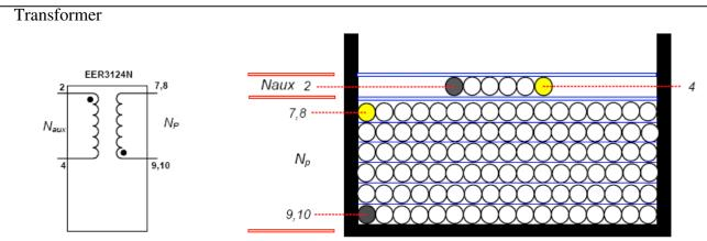
Figure 46. Transformer Schematic Diagram
