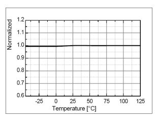
Figure 13. Current-Sense Input Threshold Voltage Limit (V<sub>CS</sub>) vs. T<sub>A</sub>
