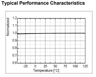
Figure 4. Voltage Feedback Input Threshold 1 (VREF1) VS. TA
