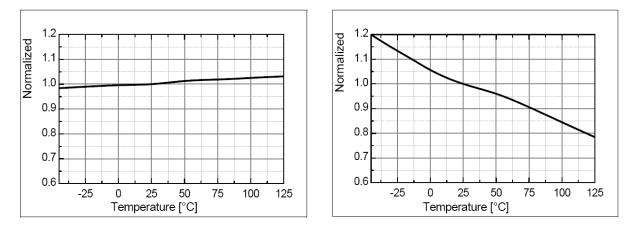
Figure 14. Input High Clamp Voltage (V<sub>CLAMPH</sub>) vs. T<sub>A</sub> Figure 15. Input Low Clamp Voltage (V<sub>CLAMPL</sub>) vs. T<sub>A</sub>
