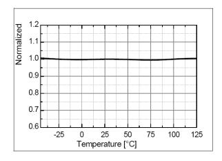
Figure 12. Maximum On-Time Program 2 (t<sub>ON,MAX2</sub>) vs. T<sub>A</sub>
