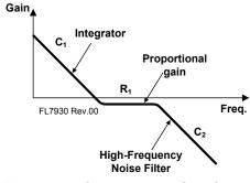
Figure 34. Compensators Gain Curve
