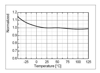
Figure 18. Restart Timer Delay (t<sub>RST</sub>) vs. T<sub>A</sub>
