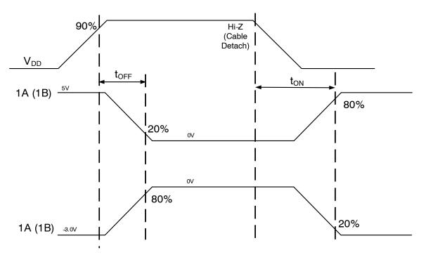
Figure 1.  $t_{\text{ON}}\,/\,t_{\text{OFF}}\,V_{\text{CC}}$  to Output Timing
