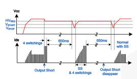
Figure 24. AOCP Waveform
