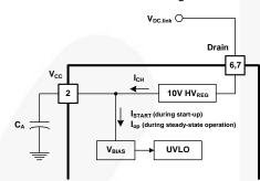
Figure 17. Startup and HV<sub>REG</sub> Block
