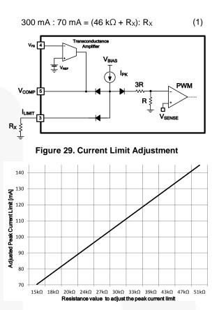
Figure 30. Current Limit vs. Rx
