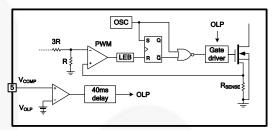
Figure 21. Overload Protection Internal Circuit
