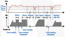
Figure 22. Overload Protection (OLP) Waveform
