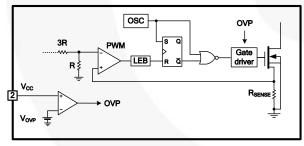
Figure 25. Over Voltage Protection Circuit
