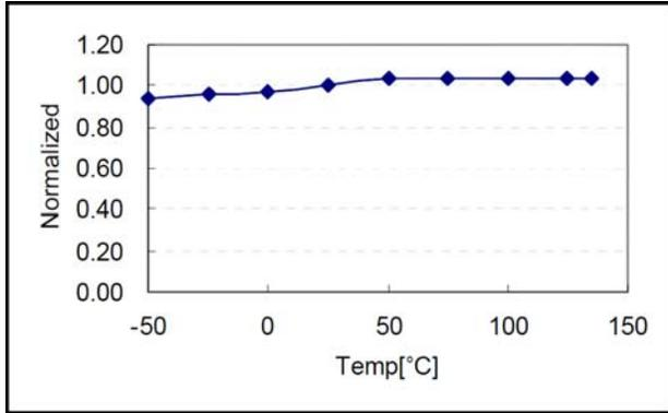
Figure 4. Operating Frequency ( $f_{osc}$ ) vs.  $T_A$
