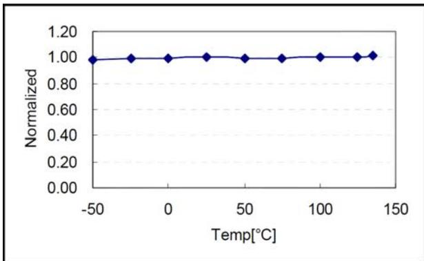
Figure 9. Stop Threshold Voltage ( $V_{STOP}$ ) vs.  $T_A$
