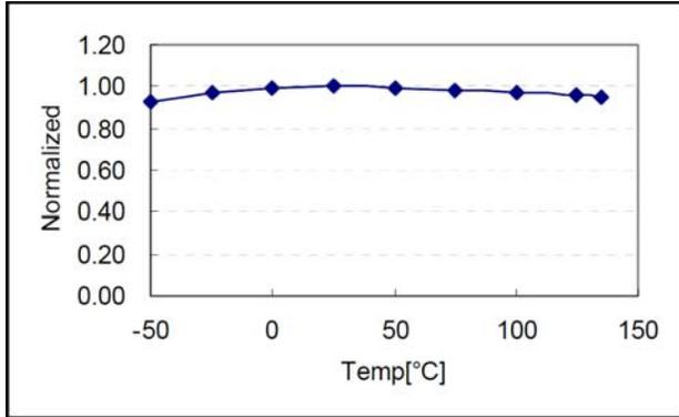
Figure 10. Feedback Source Current ( $I_{FB}$ ) vs.  $T_A$
