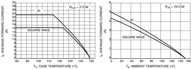
Figure 5. Current Derating, Case per Leg
