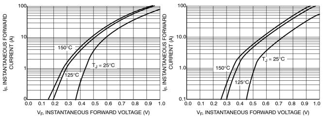
Figure 1. Typical Forward Voltage
