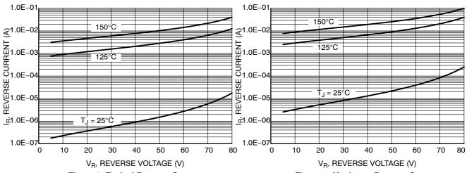
**Figure 3. Typical Reverse Current**
