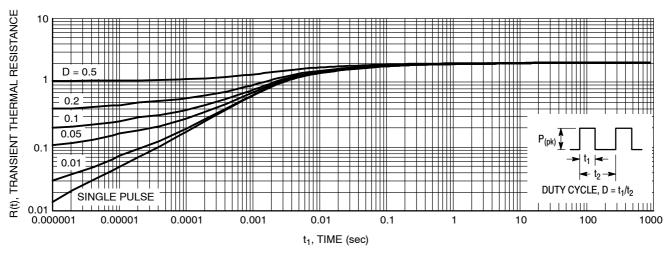
Figure 10. Thermal Response Junction-to-Case
