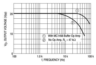
Figure 15. Large Signal Voltage versus Frequency
