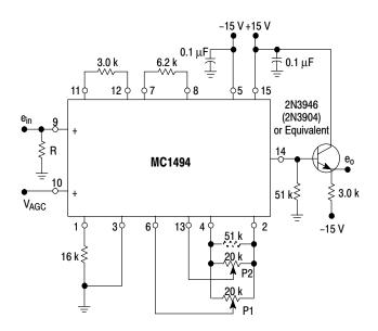
Figure 26. Wideband Amplifier with Linear AGC
