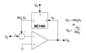
Figure 22. Basic Divide Circuit Using Multiplier
