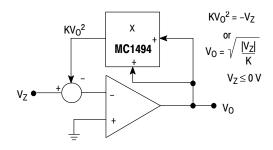
Figure 24. Basic Square Root Circuit
