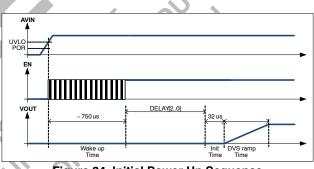
Figure 34. Initial Power Up Sequence
