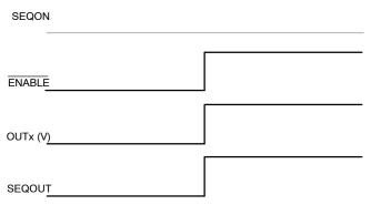
Figure 28. Sequence Interrupt from EN
