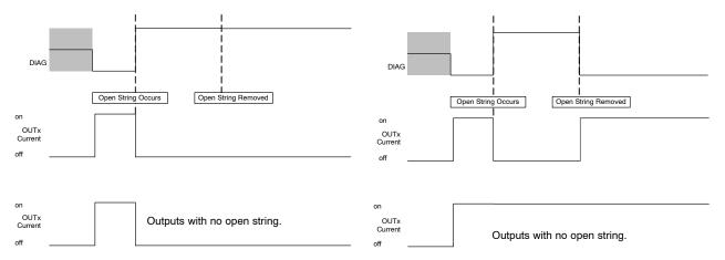
Figure 5. DIAG timing diagram WITH Open String Latch Active All outputs latch off.
