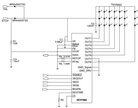
Figure 4. Application Diagram without the FET Ballast Transistor
