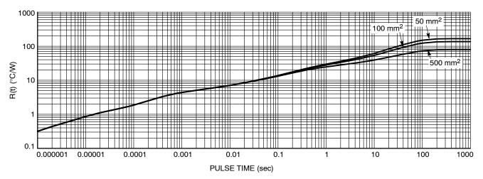
Figure 24. Single Pulse Heating Curve
