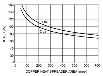
Figure 22.  $\theta_{JA}$  Copper Spreader Area
