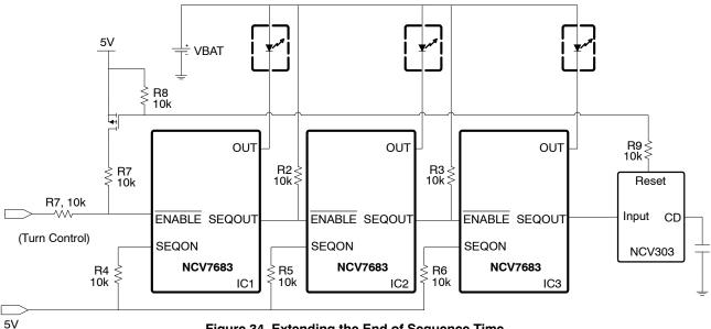
Figure 34. Extending the End of Sequence Time
