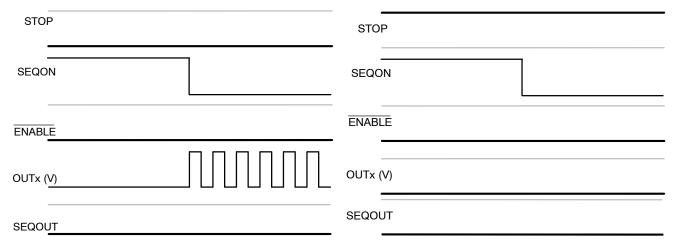
Figure 29. Sequence Interrupt from SEQON (STOP=0)
