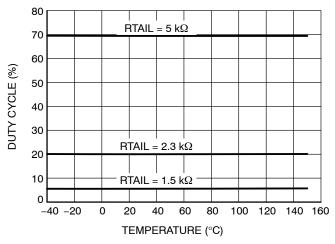
Figure 15. Duty Cycle vs. Temperature
