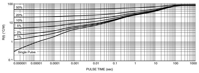
Figure 23. Thermal Duty Cycle Curves on 645 mm<sup>2</sup> Spreader Test Board
