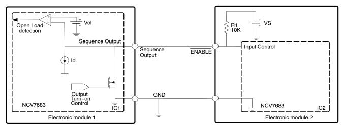
Figure 31. Daisy Chain Interface between Multiple ICs
