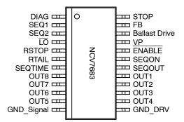
Figure 2. Pinout Diagram
