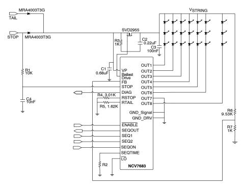
Figure 3. Application Diagram with External FET Ballast Transistor
