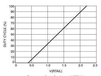
Figure 13. Duty Cycle vs. RTAIL
