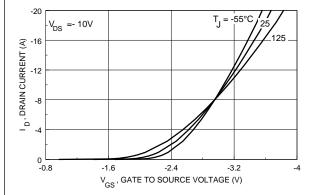
Figure 5. Transfer Characteristics.
