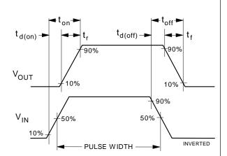
Figure 12. Switching Waveforms.
