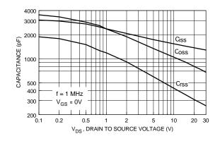
Figure 9. Capacitance Characteristics.
