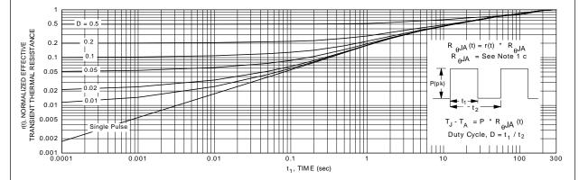
Figure 17. Transient Thermal Response Curve.
