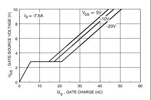
Figure 10. Gate Charge Characteristics.
