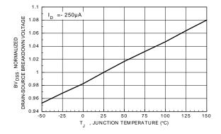
Figure 7. Breakdown Voltage Variation with Temperature.
