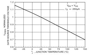
Figure 6. Gate Threshold Variation with Temperature.
