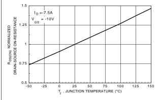
Figure 3. On-Resistance Variation with Temperature.
