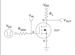
Figure 11. Switching Test Circuit.
