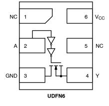
Figure 2. Pinout (Top View)
