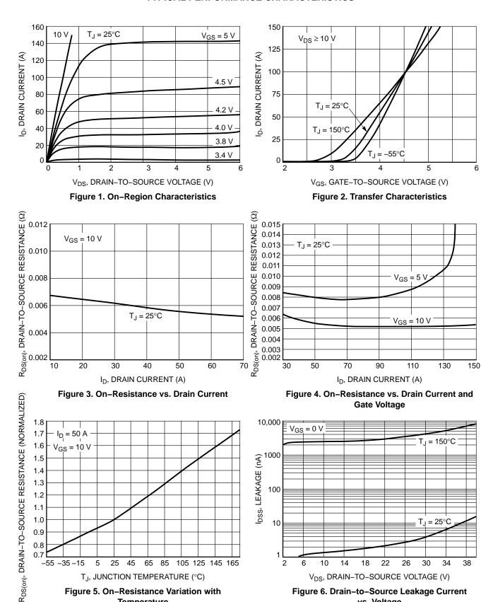
Figure 5. On-Resistance Variation with **Temperature**
