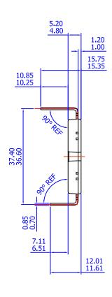
NOTES: UNLESS OTHERWISE SPECIFIED A) THIS PACKAGE DOES NOT COMPLY TO ANY CURRENT PACKAGING STANDARD B) ALL DIMENSIONS ARE IN MILLIMETERS C) DIMENSIONS ARE EXCLUSIVE OF BURRS, MOLD FLASH, AND TIE BAR EXTRUSIONS
