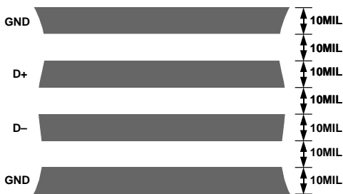
Figure 18. Arrangement of Signal Tracks
