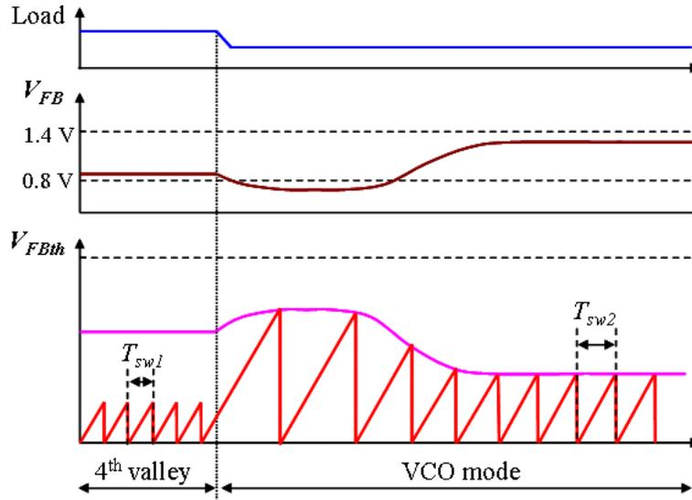
Figure 7. 4<sup>th</sup> Valley to VCO Mode Transition with an Optimum Timing Capacitor C<sub>t</sub>
