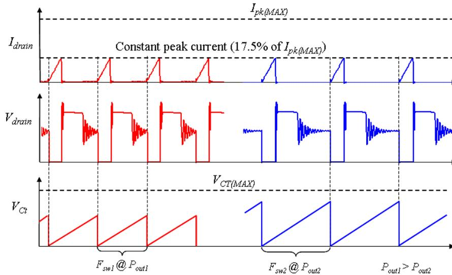
Figure 5.  $I_{drain}$ ,  $V_{drain}$ ,  $V_{ct}$ , at Different Output Loads in VCO Mode
