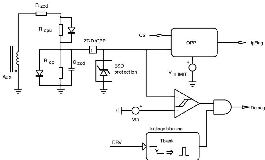
**Figure 9. ZCD and OPP Circuit**
