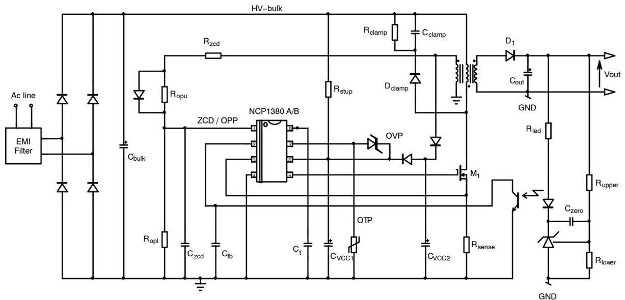
Figure 1. Application Schematic for Versions A and B
