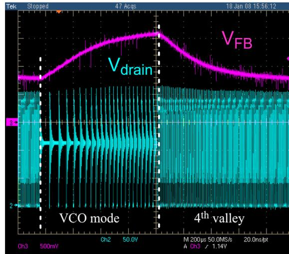
Figure 6. The Controller Hesitates Between VCO Mode and 4<sup>th</sup> Valley:  $C_t$  is Too Big!
