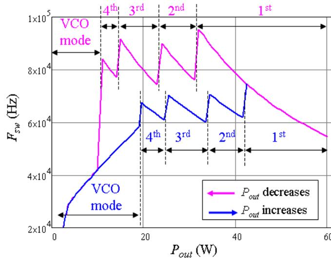
Figure 4. Switching Frequency versus Output Power at  $V_{in} = 90 \text{ Vrms}$
