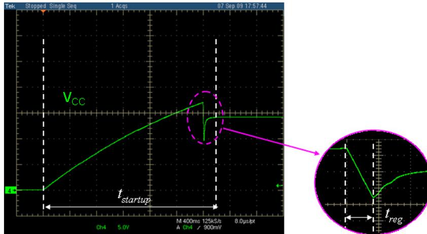
**Figure 11.  $V_{CC}$  Waveform During Startup**
