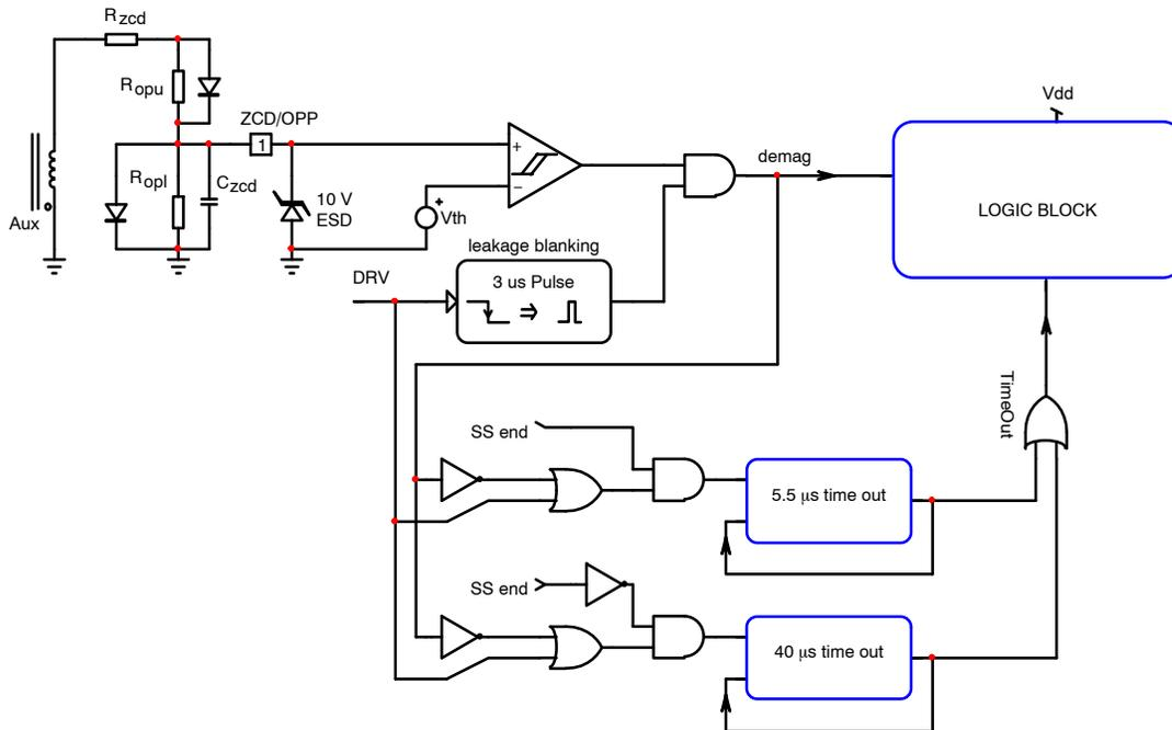
Figure 8. Zero-Crossing Detection Bloc Schematic
