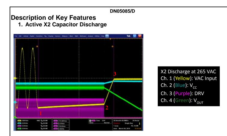
The NCP1340 features integrated active input filter (X2) capacitor discharge, eliminating the need for external discharge resistors which are major contributors to the total power dissipation in light load and standby mode operation. The integrated discharge circuit is virtually lossless across all operating modes and only consumes power when it is needed to discharge the X2 capacitors.
