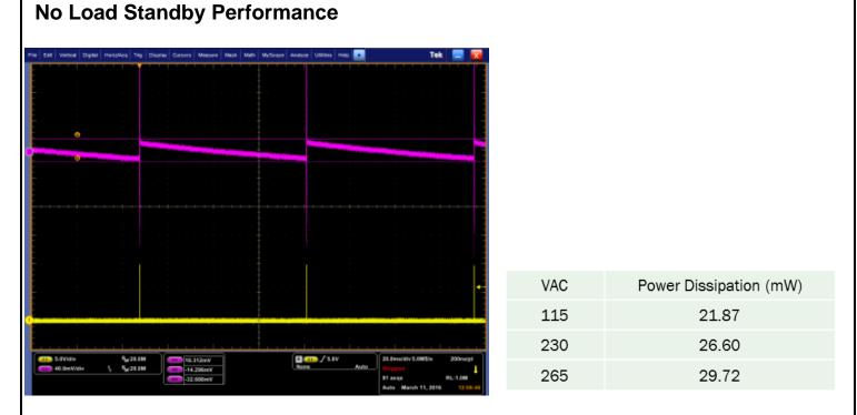
The NCP1340 features low current consumption when operating in a burst mode to enable very low no load standby power operation. In no load, the system was able to achieve less than 30 mW of power dissipation across the line operating range meeting CoC Tier II and DoE requirements. The output voltage ripple while in no load was  $\sim$  33 mV.
