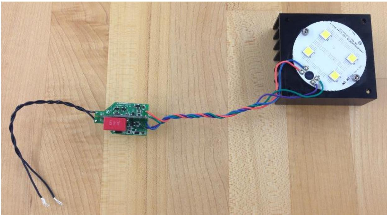
Figure 1 – Evaluation board with heat sink for LEDs.
