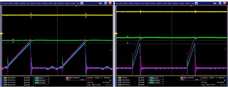
**Figure 6: Over Power Protection Waveform**
