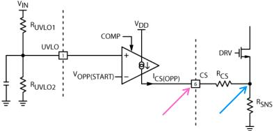
Figure 5: Over Power Protection Circuit
