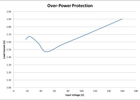
Figure 7: Overload Current vs Input Voltage
