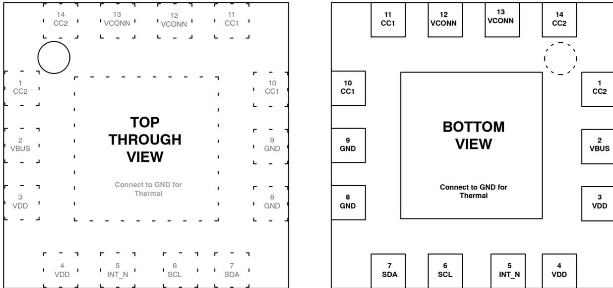
Figure 5. FUSB302BMPX Pin Assignment (N/C = No Connect)
