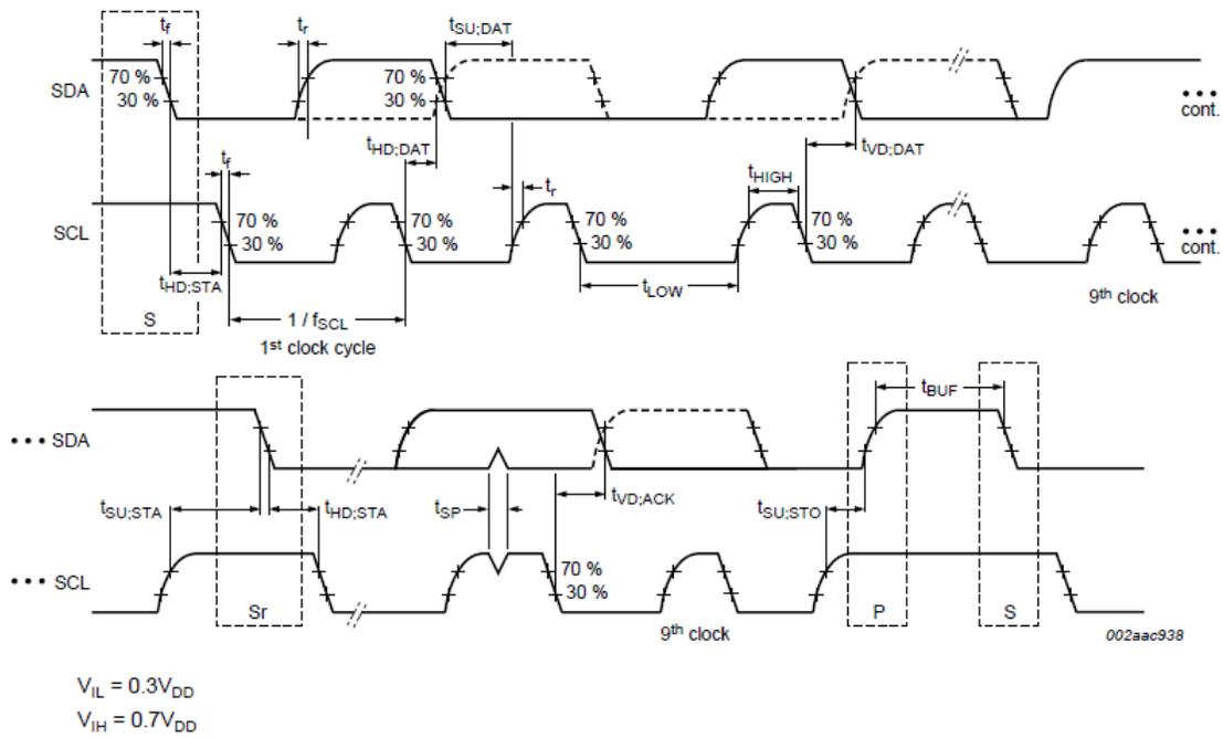
Figure 17. Definition of Timing for Full-Speed Mode Devices on the I<sup>2</sup>C Bus
