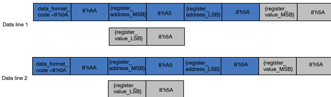
Figure 16. Format of Embedded Data Output within a Frame
