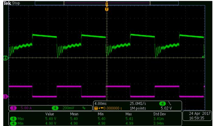
Test condition: 0-4A, 10ms cycle and 250mA/us, 115Vac
