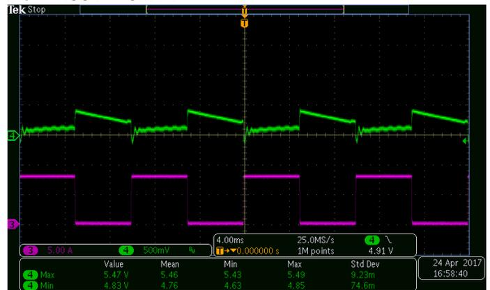
Test condition: 0.1A-8A, 10ms cycle and 250mA/us, 115Vac
