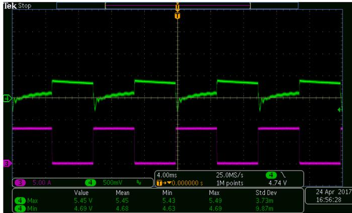
Test condition: 0-8A, 10ms cycle and 250mA/us, 115Vac
