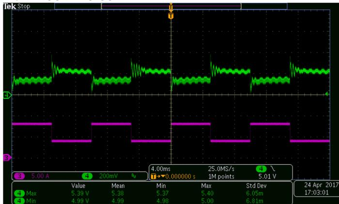
Test condition: 4-8A, 10ms cycle and 250mA/us, 115Vac
