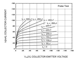
Figure 1. Static Characteristic
