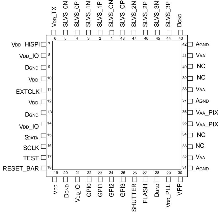
Figure 7. 48-Pin ILCC HiSPi Package Pinout Diagram
