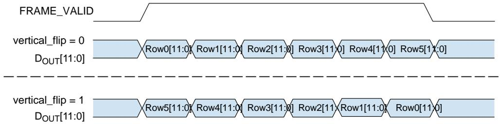
**Figure 29. Effect of Vertical Flip on Readout Order**
