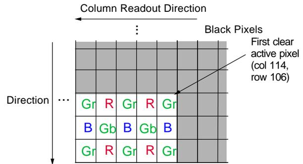
Figure 3. Pixel Color Pattern Detail (Top Right Corner)
