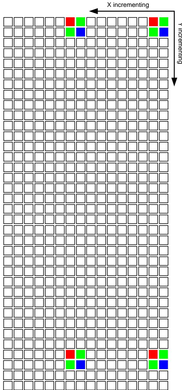
**Figure 38. Pixel Readout (x\_odd\_inc = 7, y\_odd\_inc = 31)**
