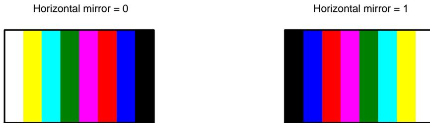
Figure 56. 100% Color Bars Test Pattern
