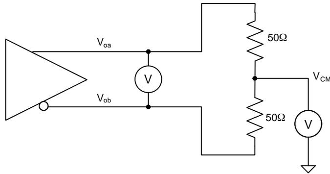
Figure 70. DC Test Circuit
