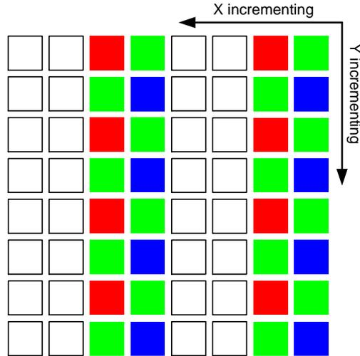
Figure 33. Pixel Readout ( $x\_odd\_inc = 3$ ,  $y\_odd\_inc = 1$ )
