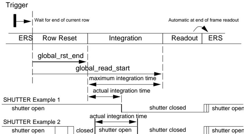
Figure 49. Control of the Electromechanical Shutter
