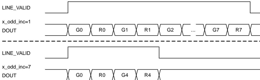
**Figure 31. Effect of x\_odd\_inc = 7 on Readout Sequence**
