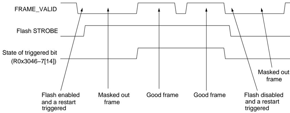
**Figure 45. LED Flash Enabled Following Forced Restart**
