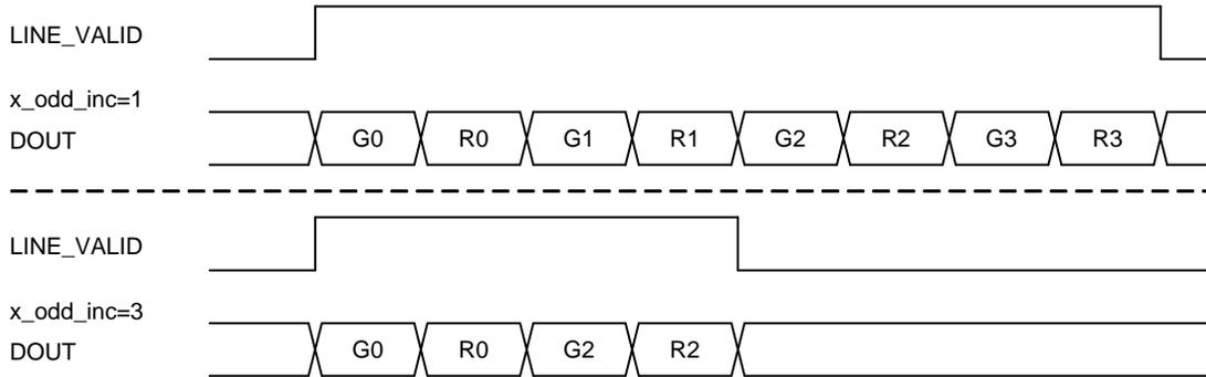
**Figure 30. Effect of x\_odd\_inc = 3 on Readout Sequence**
