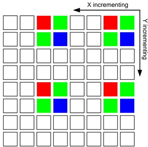
Figure 35. Pixel Readout ( $x\_odd\_inc = 31, y\_odd\_inc = 3$ )
