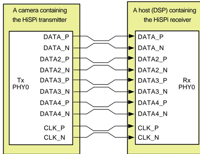
Figure 10. HiSPi Transmitter and Receiver Interface Block Diagram
