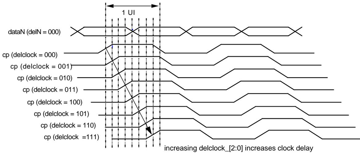
Figure 13. Delaying the clock\_lane with Respect to data\_lane
