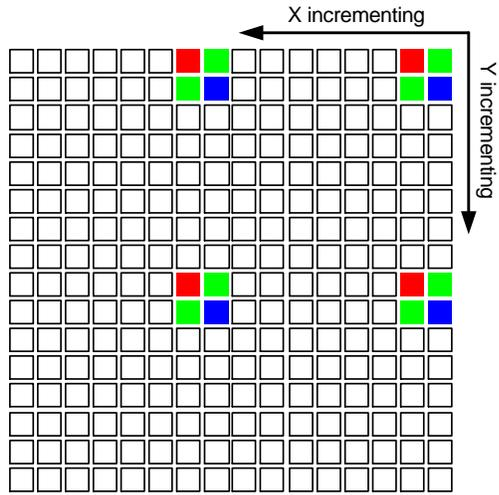
Figure 36. Pixel Readout ( $x\_odd\_inc = 7, y\_odd\_inc = 7$ )
