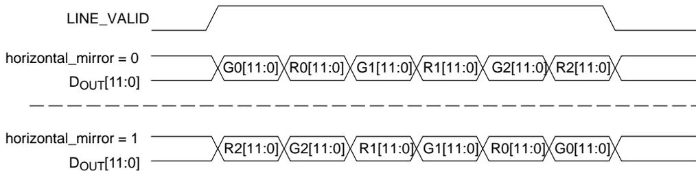
**Figure 28. Effect of Horizontal Mirror on Readout Order**
