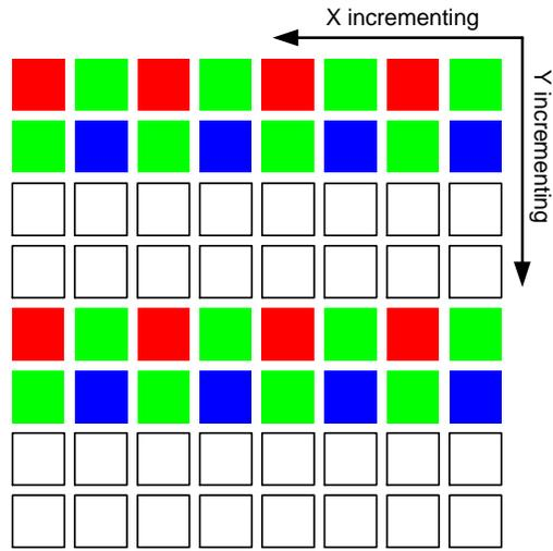
Figure 34. Pixel Readout ( $x\_odd\_inc = 1, y\_odd\_inc = 3$ )
