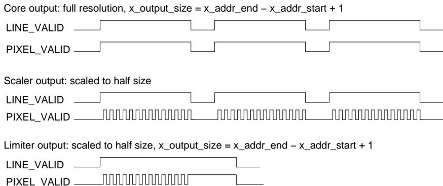
**Figure 24. Effect of Limiter on the Data Path**
