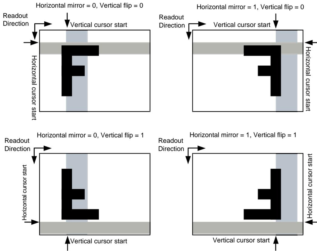
Figure 61. Test Cursor Behavior with Image Orientation
