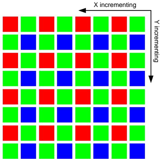
Figure 32. Pixel Readout (No Subsampling)
