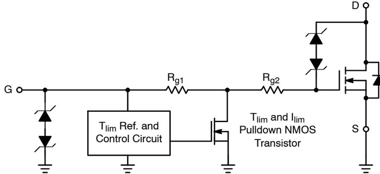
Figure 4. Simplified Input Circuit
