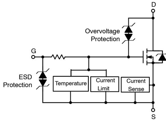
Figure 2. Generic Block Architecture of Low Side SmartFETs
