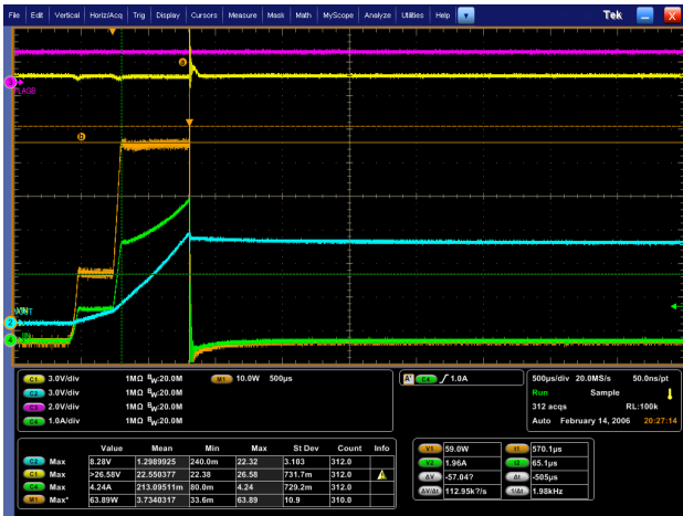
Figure 4. V_{IN} = 22\text{ V} , C_{SS} = 5.6\text{ nF} , C_{IN} = 10\text{ }\mu\text{F} , C_{OUT} = 280\text{ }\mu\text{F}
