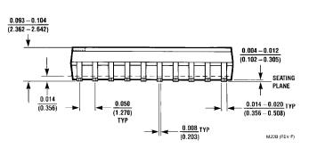
Figure 4. 20-Lead Small Outline Integrated Circuit (SOIC), JEDEC MS-013, 0.300" Wide Package Number M20B
