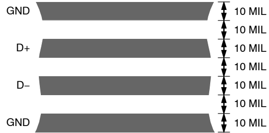
Figure 18. Arrangement of Signal Tracks
