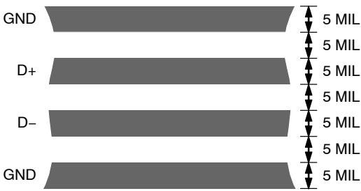
Figure 21. Typical Arrangement of Signal Tracks
