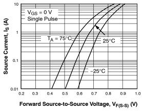
Figure 6. Forward Source-to-Source Voltage vs. Current
