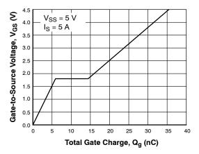
Figure 8. Gate-to-Source Voltage vs. Total Charge
