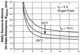
Gate-to-Source Voltage, V<sub>GS</sub> (V)
