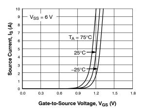
Figure 3. Transfer Characteristics
