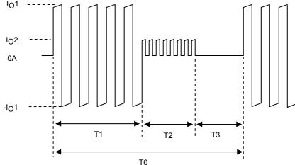
Figure 1 Motor Current Timing
