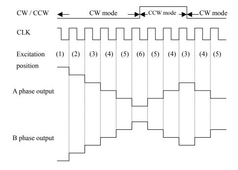
The internal D/A converter proceeds by a bit on the rising edge of the step signal input to the CLK pin. In addition, CW and CCW mode are switched by CW and CCW pin setting.
