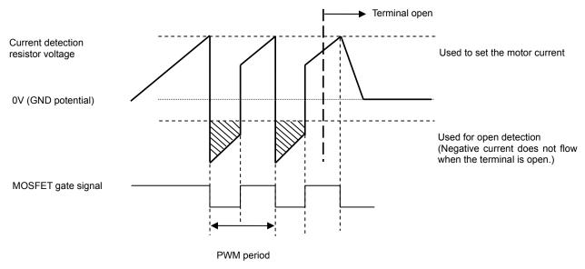
When the current level drops, the difference with the GND potential decreases, making detection difficult. The motor current that can be detected by motor terminal open detection is 1.1A or more with the STK672-432BN-E and 1.4A or more with the STK672-440BN-E/442BN-E.
