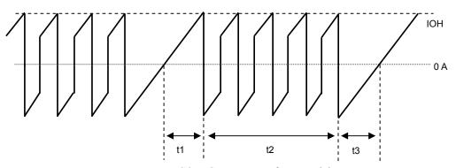
Motor COM Current Waveform Model
