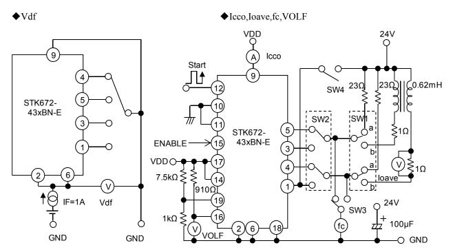
Ioave measurement: Set switch SW2 in the setting SW1 to 'b'.
