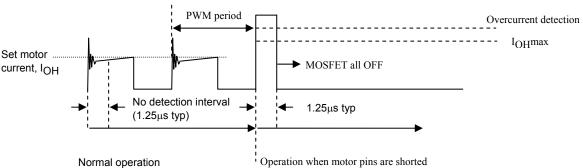
Overcurrent detection begins after an interval of no detection (a dead time of  $1.25\mu s$  typ) during the initial ringing part during PWM operations. The no detection interval is a period of time where overcurrent is not detected even if the current exceeds IOH.
