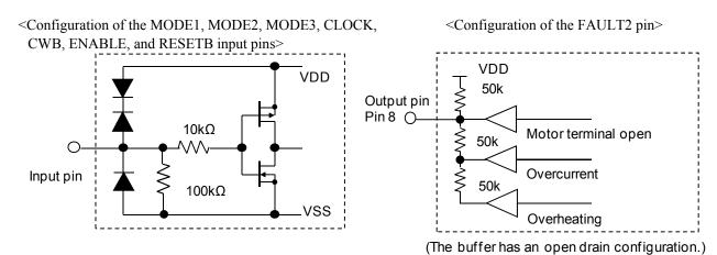
The input pins of this driver all use Schmitt input. Typical specifications at Tc=25°C are given below. Hysteresis voltage is 0.3V (VIHa-VILa).
