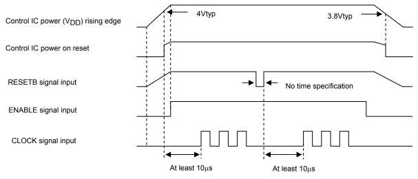
ENABLE, CLOCK, and RESETB Signals Input Timing
