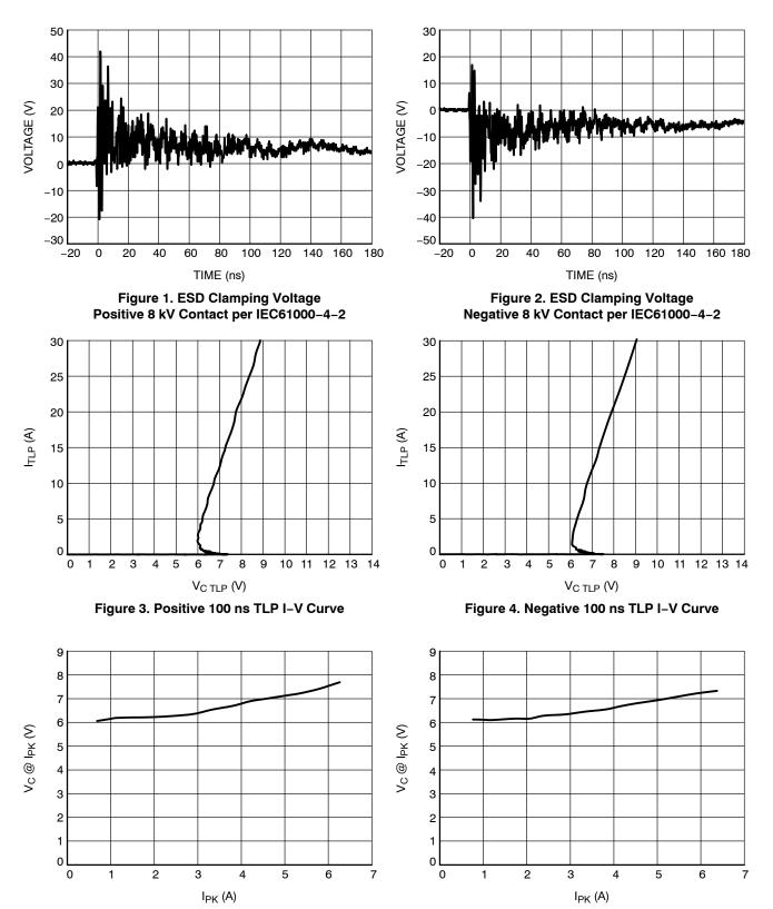
Figure 5. Clamping Voltage vs. Peak Pulse Current – Pin 1 to Pin 2 (tp =  $8/20 \mu s$ )
