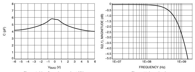
Figure 9. Line Capacitance, f = 1 MHz
