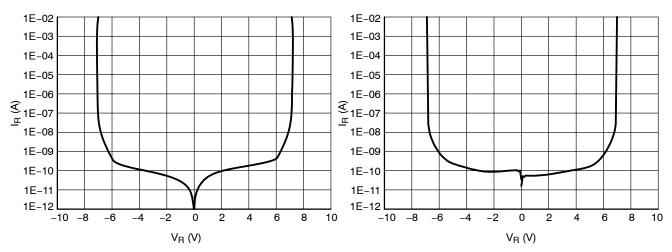
Figure 7. Breakdown Voltage
