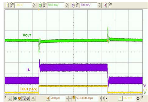
图 19. 负载瞬态, 200–800–200 mA, 100 ns 边沿
