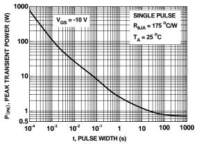
Figure 12. Single Pulse Maximum Power Dissipation
