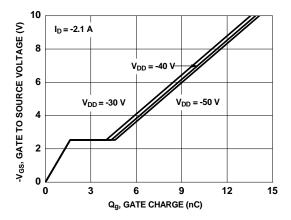
Figure 7. Gate Charge Characteristics
