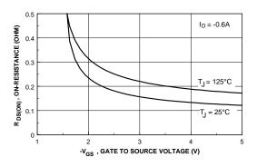
Figure 4. On-Resistance Variation with Gate-to-Source Voltage.
