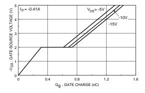
Figure 17. Gate Charge Characteristics.
