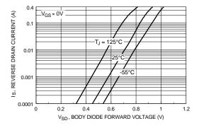
Figure 6. Body Diode Forward Voltage
