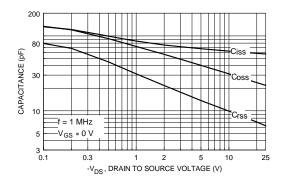
Figure 18. Capacitance Characteristics.
