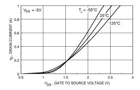
Figure 15. Transfer Characteristics.
