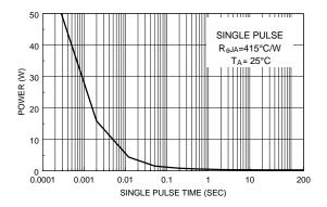
Figure 10. Single Pulse Maximum Power Dissipation.
