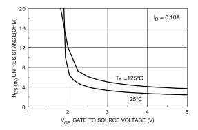
Figure 4. On-Resistance Variation with Gate-to-Source Voltage.
