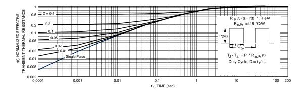
Figure 21. Transient Thermal Response Curve.
