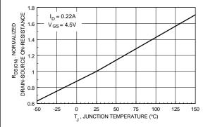
Figure 3. On-Resistance Variation with Temperature.
