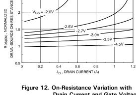
Drain Current and Gate Voltage.
