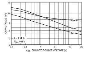
Figure 8. Capacitance Characteristics.
