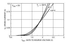
Figure 5. Transfer Characteristics.
