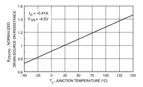
Figure 13. On-Resistance Variation with Temperature.
