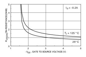
Figure 14. On-Resistance Variation with Gate-to-Source Voltage.
