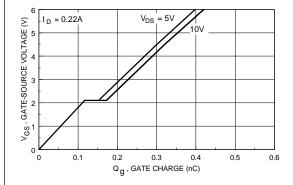
Figure 7. Gate Charge Characteristics.
