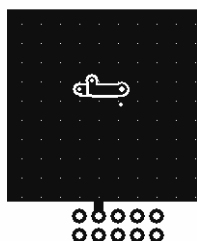
a. 53^\circ\text{C/W} when mounted on a 1 in 2 pad of 2 oz copper
